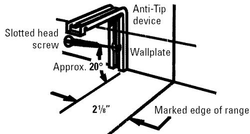
B. Locate the outside edge of the device  $2\frac{1}{8}$ " toward the center of the range from the marked edge of the range.
