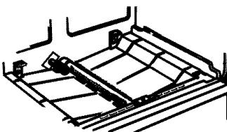
To determine if the bottom burner flames are burning properly, remove the oven bottom. Flames should have approximately 1" blue cones and, if range is supplied with natural gas, should burn with no yellow tipping. (With most LP gas, small yellow tips at the end of outer cones are normal.) Flames should not lift off burner ports. If lifting is observed, gradually reduce air shutter opening until flames are stabilized.
