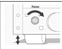
All four corners of your refrigerator must rest firmly on a solid floor. Your refrigerator is equipped with adjustable front rollers to help level your unit. To ensure proper door seal and assist door closing, the refrigerator should be tilted 1/4" (6 mm), front to back.
