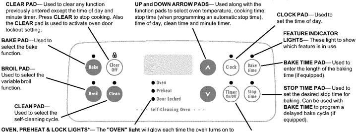
maintain set oven temperature. The "PREHEAT" light will glow when the oven is first set to operate, TIMER PAD—Used to set or cancel the minute or if the desired temperature is reset higher than the actual oven temperature. The "DOOR LOCKED" light will flash when the oven door locks & unlocks or when using the self-clean cycle or the oven door lockout mode is activated. The indicator light will glow constantly after the door locks.
