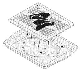
The broiler pan with the insert allows grease to drain and be kept away from the high heat of the broiler. **DO NOT** use the pan without the insert. **DO NOT** cover the insert with foil. The exposed grease could ignite.
