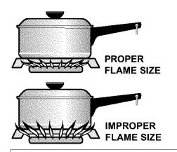
Never extend the flame beyond the outer edge of the utensil. A higher flame simply wastes heat and energy, and increases your risk of being burned by the flame.
