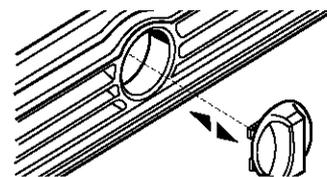
3. Rotate the cartridge cap to a horizontal position. The cartridge cap might not be even with the base grille.
