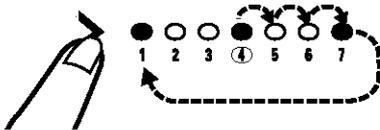
**NOTE:** With each press of the arrow, you will hear a beep as the light moves to the next setting. The indicator light moves to a setting of “7” and then returns to the setting of “1”.
