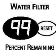
After changing the water filter cartridge, reset the water filter status light by pressing and holding the RESET for 2 seconds. The indicator light will change to 99% when the filter indicator is reset.
