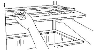
3. Replace back of meat drawer cover frame into supports or slides on side walls of the refrigerator and lower or slide the front of the cover frame into place.
