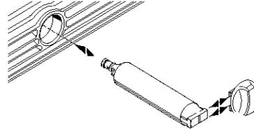
3. Take the new cartridge out of its packaging and remove protective cover from o-rings.
