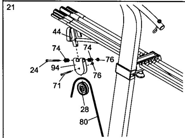
Wrap the Long Cable (80) around a 90mm Pulley (28). Attach the Pulley inside of the Pulley Housing (94) with an M10 x 42mm Button Head Bolt (71) and an M10 Nylon Locknut (76).
