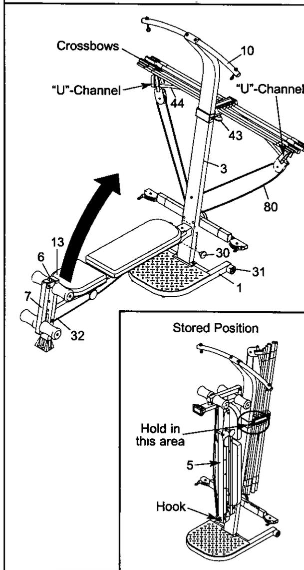
**⚠ WARNING:** Be sure that all of the crossbows are removed from the "U"-channels before moving the crossbow assembly to the stored position.
