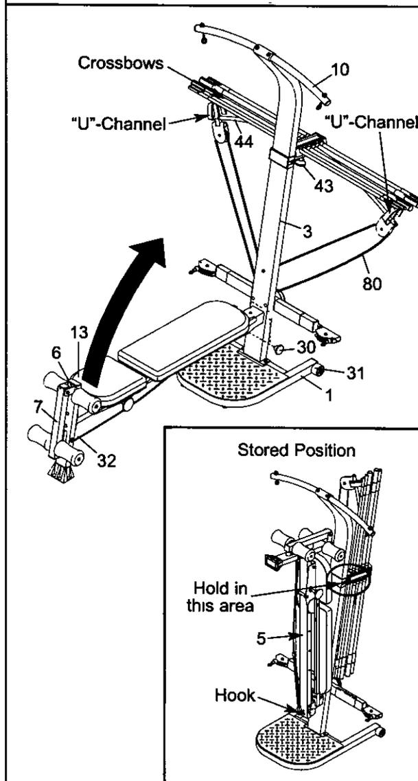
**WARNING:** Be sure that all of the crossbows are removed from the "U"-channels before moving the crossbow assembly to the stored position.
