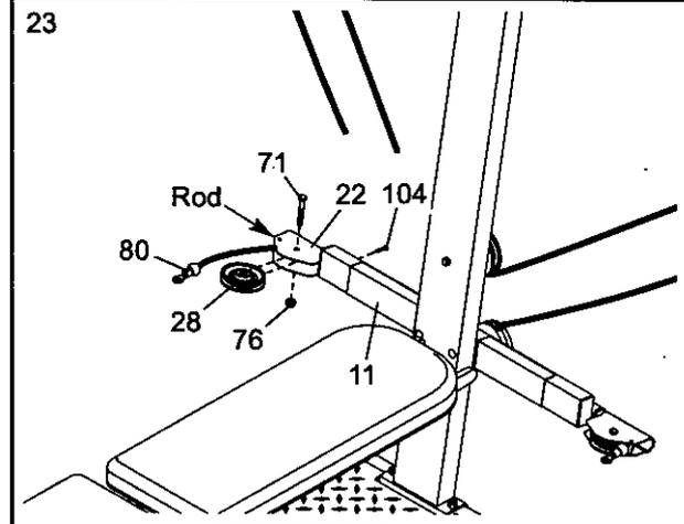
Insert the end of the Long Cable (80) through the welded tube on the indicated end of the Cross Tube (11) and then through the remaining Swivel Arm (22). **Be sure the Cable is on the indicated side of the welded rod in the Swivel Arm.**
