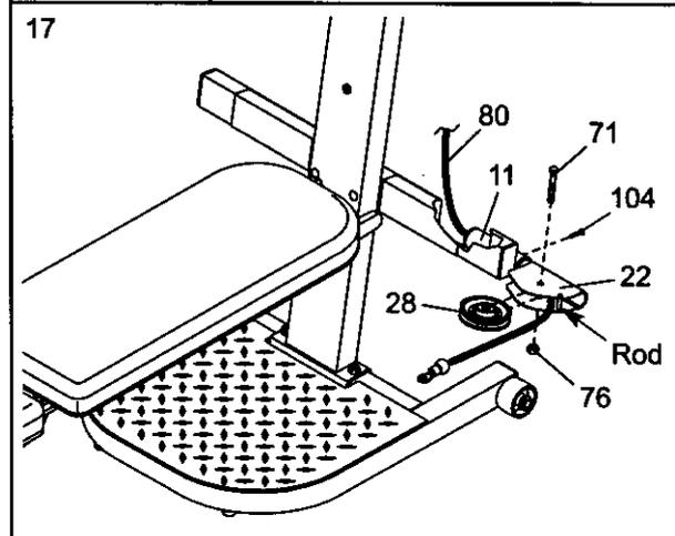
18. Wrap the Long Cable (80) around a 90mm Pulley (28). Attach the Pulley and a Pulley Guard (29) to the indicated M10 x 140mm Carriage Bolt (73) with an M10 Nylon Locknut (76). **Be sure the flat edge of the Pulley Guard is on the side shown.**
