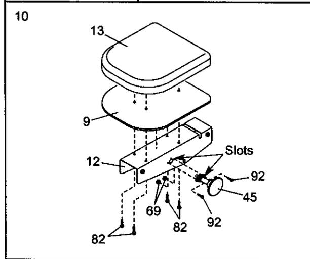
11. Pull out the Seat Knob (45) as far as it will go, and set the Seat Carriage (12) on the Bench Rail (5).
