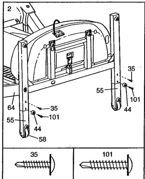
3. With the help of a second person, carefully tip the Uprights (64) back to the vertical position.
