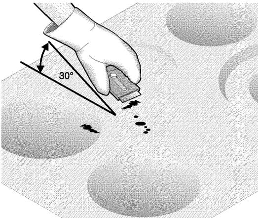
If soils remain, carefully scrape soils with a metal razor blade scraper, holding scraper at a 30 degree angle to the surface. Remove loosened soils with cooktop cleaning cream and buff surface clean.
