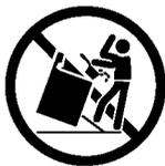
**⚠ WARNING** Stepping, leaning or sitting on the doors or drawers of this range can result in serious injuries and also cause damage to the range. Do not allow children to climb or play around the range. The weight of a child on an open door may cause the range to tip, resulting in serious burns or other injury.
