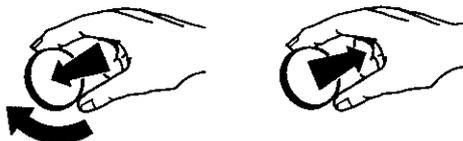
Pull out the Cycle Control knob to start the washer.
