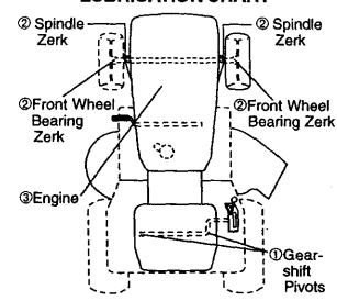
**①SAE 30 or 10w30 MOTOR OIL** *QGENERAL PURPOSE GREASE* **③REFER TO Maintenance "ENGINE" SECTION IMPORTANT:** Do not oil or grease the pivot points which have special nylon bearings. Viscous lubricants will attract dust and dirt that will shorten the life of the self-lubricating bearings. If you feel they must be lubricated, use only a dry, powdered graphite type lubricant sparingly.
