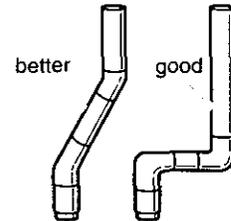
5. Use duct tape to seal all joints. **Do not** use screws to secure vent. Lint may catch on screws.
