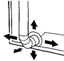
4. Use the straightest path possible when routing the exhaust vent. Use the fewest number of elbows and turns. Allow room when using elbows or making turns. Bend vent gradually to avoid kinking.
