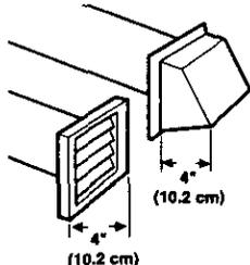
3. The exhaust vent can be routed up, down, left, right, or straight out the back of the dryer. Space requirements are listed in your Installation Instructions.
