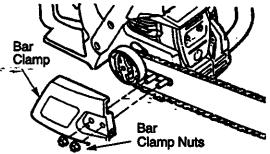
• Turn adjusting screw on bar to move the tensioning rack as far as it will go toward the front of the bar.
