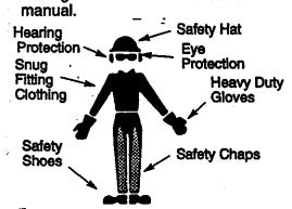
Wear protective gear. Always use steel-toed safety footwear with nonslip soles; snug-fitting clothing; heavyduty, non-slip gloves; eye protection such as non-fogging, vented goggles or face screen; an approved safety hard hat; and sound barriers (ear plugs or mufflers) to protect your hearing. Regular users should have hearing checked regularly as chain saw noise can damage hearing. Secure hair above shoulder length.
