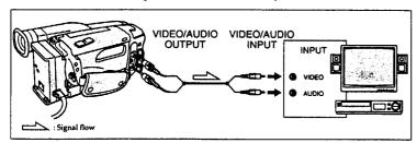
To connect a TV or a VCR without Video/Audio input jacks Use the RFU-95UC RFU adaptor (not supplied).
