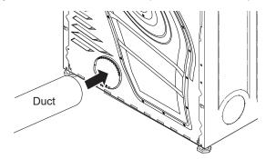
**NOTE:** We strongly recommend using rigid metal exhaust duct. However, if flexible ducting is used it must be UL-Listed metal, not plastic.
