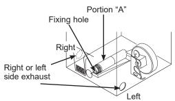
Reconnect the cut portion (A) of the duct to the blower housing. Make sure that the shortened duct is aligned with the tab in the base. Use the screw saved previously to secure the duct in place through the tab on the appliance base.
