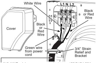
4 #10 AWG minimum copper conductors or 120/240V 30A power supply cord kit marked for use with dryers and provided with closed loop or spade terminals with upturned ends (not supplied).
