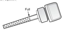
4. If needed, slowly pour oil into oil fill opening to the full mark on dipstick. Do not overfill.
