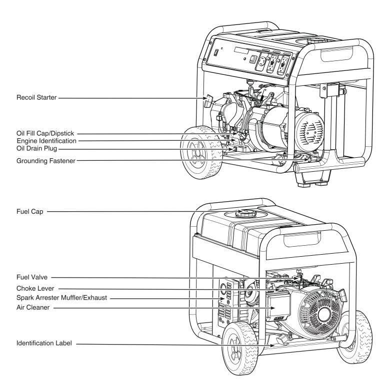
Air Cleaner — Filters engine intake air.
