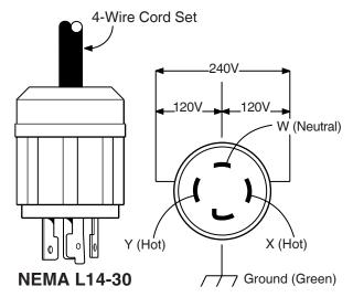
This receptacle powers 120/240 Volt AC, 60 Hz, single phase loads requiring up to 6,250 Watts of power (6.25 kW) at 26.0 Amps for 240 Volts or two independent 120 Volt loads at 26.0 Amps each.
