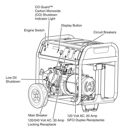
120 Volt AC, 20 Amp, GFCI Duplex Receptacles — Used to supply 120 Volt AC, single phase, 60 Hz power for electrical lighting, appliance, tool and motor loads.
