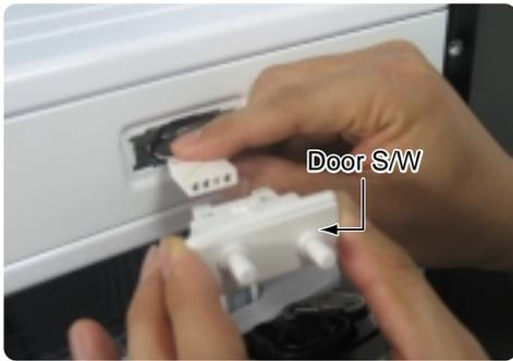
13. Disassemble the Cap Door S/W, Sleeve and the screws.
