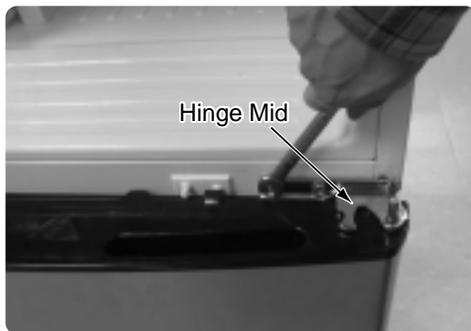
7. Disassemble the Freezer Door by lifting it upward.
