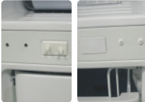
15. Assemble Freezer Door by fitting Hinge-Low into the grommet hinge hole. Don't forget to insert washer with grease.
