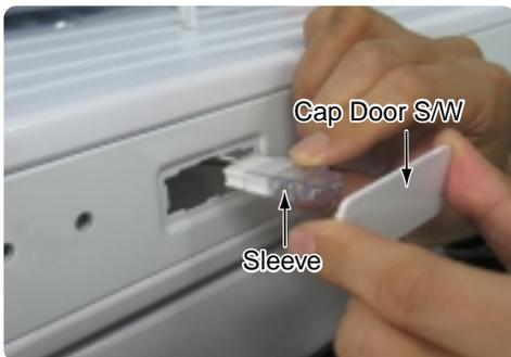
14. Assemble the each part into the reverse side as below picture. Assemble the Door S/W as it is. (Make sure not to insert it upside down)
