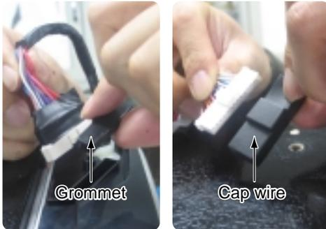
24. Assemble the parts to the reverse side. Electric wires must be sealed in covers.
