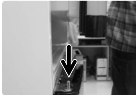
22. After removing the screw, disassemble the Cover-Cap Door and Cover Hinge.
