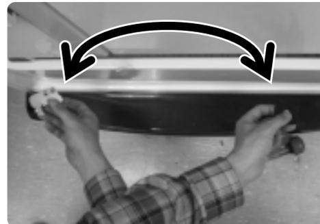
10. After removing the left and right side screws, disassemble the Grommet, Stopper Door and Stopper-Mid of the right bottom of freezer-door.
