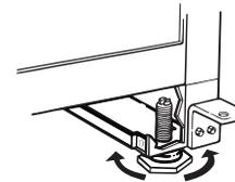
5. Push up on the top rear of the ice maker and locate the leveling legs that are on the bottom rear of the ice maker.
