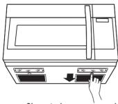
3. Soak grease filters in hot water and a mild detergent. Scrub and swish to remove embedded dirt and grease. Rinse well and shake to dry. Do not clean filters with ammonia, corrosive cleaning agents, such as lye-based oven cleaners, or place them in a dishwasher. The filters will turn black or become damaged.
