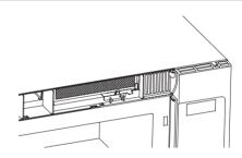
9. Reinstall the vent by sliding the bottom of the vent into place. Push the vent top into position and slide right until it snaps into place. Replace the two vent mounting screws located on top of the microwave using a #1 Phillips screwdriver.
