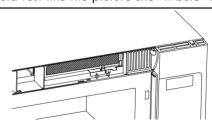
6. Reinstall the vent by sliding the bottom of the vent into place. Push the vent top into position and slide right into place. Replace the two vent mounting screws located on top of the microwave using a #1 Phillips screwdriver.
