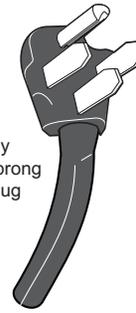
Power supply cord with 4-prong grounding plug
