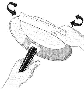
Figure 1: Check pan for flat bottom using ruler
