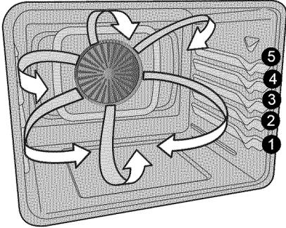
Figure 19: Air circulation in the convection roast
