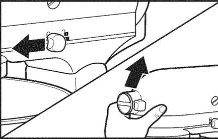
**1 To lift motor head:** Push the locking lever to the UNLOCK position and lift the head. Once lifted, the lever will automatically go back in LOCK position to keep the head lifted.
