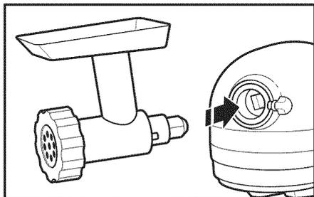
**3** Insert attachment shaft housing into attachment hub, making certain that attachment power shaft fits into square attachment hub socket. It may be necessary to rotate attachment back and forth. When attachment is in proper position, the pin on the attachment will fit into the notch on the hub rim.
