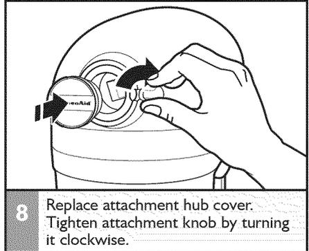
**8** Replace attachment hub cover. Tighten attachment knob by turning it clockwise.
