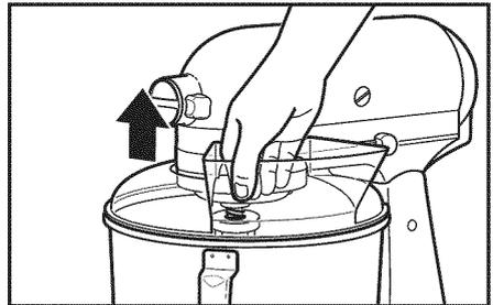
**4** Lift the front of the pouring shield clear of the bowl rim and pull forward. Remove attachment and bowl.
