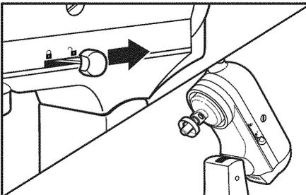
**2 Hold the locking lever in the UNLOCK position and tilt motor head back.**
