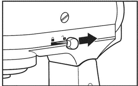
**2 To put down motor head:** Push the locking lever to UNLOCK and gently bring the head down. The locking lever will automatically go back in LOCK position when the head is down. Before mixing, test lock by attempting to raise motor head.
