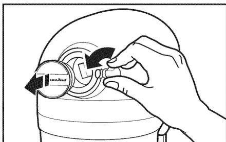
**2** Loosen attachment knob by turning it counterclockwise. Remove attachment hub cover.
