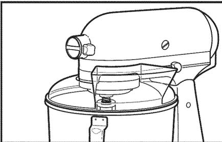
**1** For best results, rotate the shield so the motor head covers the U-shaped gap in the shield. The pouring chute will be just to the right of the attachment hub as you face the Stand Mixer.
