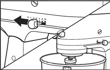
**1 To place pouring shield:** Turn speed control to “0”. Unplug Stand Mixer. Attach your chosen accessory, see “Attaching/removing the flat beater, wire whip, or dough hook” section.
