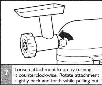
**7** Loosen attachment knob by turning it counterclockwise. Rotate attachment slightly back and forth while pulling out.
