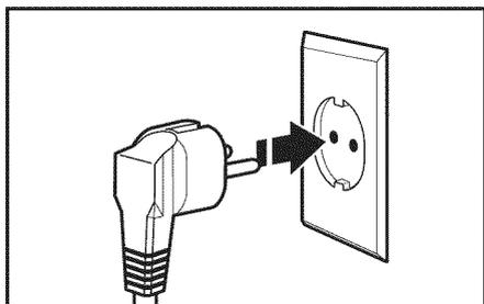
**5** Plug into proper electrical outlet.
