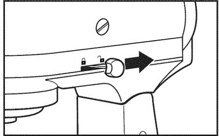
**2 To put down motor head:** Push the locking lever to UNLOCK and gently bring the head down. The locking lever will automatically go back in LOCK position when the head is down. Before mixing, test lock by attempting to raise motor head.
