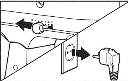
**3 To Remove pouring shield:** Turn speed control to “0”. Unplug Stand Mixer.
