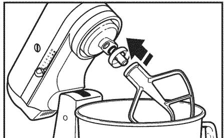
**3 Slip accessory onto beater shaft and press upward as far as possible. Then, turn accessory to the right, hooking accessory over the pin on the shaft.**
