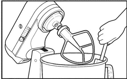
**2** Do not scrape bowl while Stand Mixer is operating. The bowl and beater are designed to provide thorough mixing without frequent scraping. Scraping the bowl once or twice during mixing is usually sufficient.
