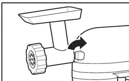
**4** Tighten attachment knob by turning clockwise until attachment is completely secured to Stand Mixer.
