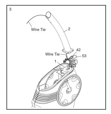
4. **Tip: Avoid pinching the wires.** Set the Upright (2) on the Frame (1).
