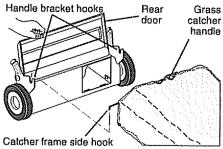
For DOOR PIVOT PIN mounted catcher, place the grass catcher frame hooks onto the door pivot pins.
