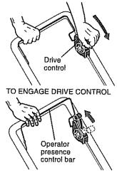
DRIVE CONTROL DISENGAGED
