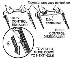
Over time, the drive control system may become "loose", resulting in decreased speed. There are holes in the drive control housing to increase tension on the drive cable. Proceed as follows:
