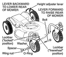
CASTER WHEEL OPERATION ("THREE POINT" ADJUSTMENT ONLY) The front wheels can be "locked" into position or set to "freewheel" for better maneuverability. Placing the lockbars in the outer holes of the adjustment brackets "locks" the front wheels. Likewise, placing the lockbars in the inner holes of the adjustment brackets allows the front wheels to spin freely ("freewheel").
