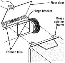
For HANDLE BRACKET mounted catcher, place frame side hooks into slots in handle brackets.
