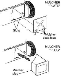
MULCHER PLUG BUILT INTO REAR DOOR
