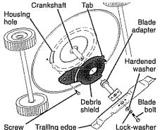
Use a wood block between blade and mower housing to prevent blade from turning when removing blade bolt.
