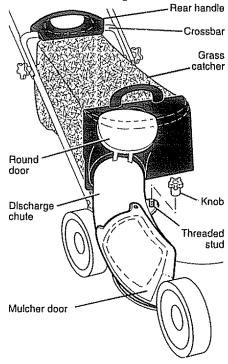
Open mulcher door and insert tabs of discharge chute into hinge bracket opening and position rear of chute over threaded stud.
