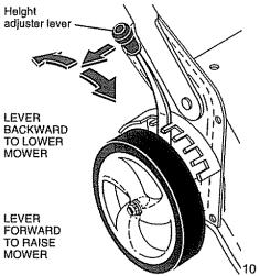
"THREE POINT" ADJUSTMENT (18" (45cm) HI-VAC MODELS ONLY) Both rear wheels are adjusted by a single lever on the left rear wheel
