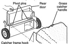
For DOOR SLOT mounted catcher, place the grass catcher frame hooks into the slots of the rear door.
