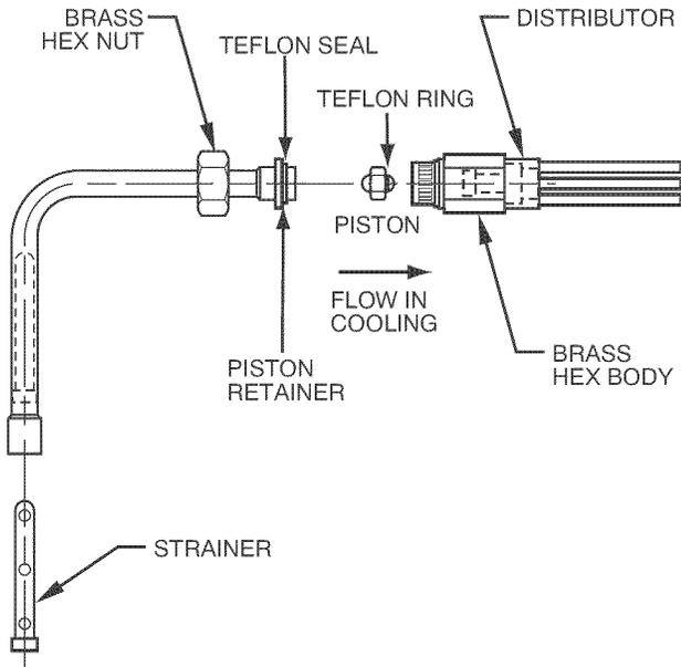
Fig. 19 - Refrigerant Flow - Control Device
