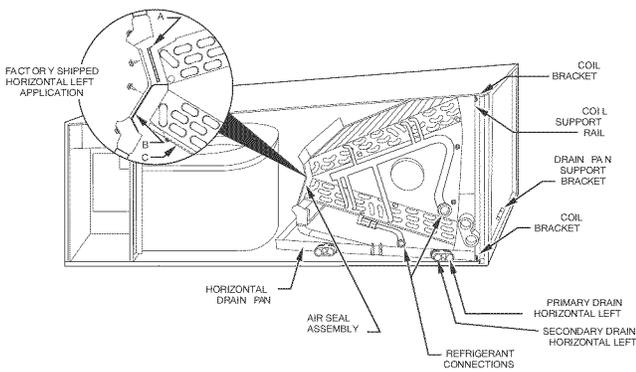
**Fig. 3 - A-Coil in Horizontal Left Application (Factory Ready)**
