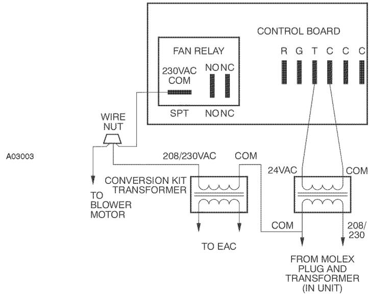
**Fig. 23 - Wiring Layout of Electronic Air Cleaner to Fan Coil for FY5B Models Only**
