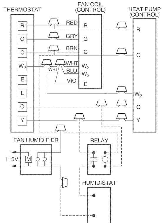
**Fig. 24 - Wiring Layout of Humidifier to Heat Pump**
