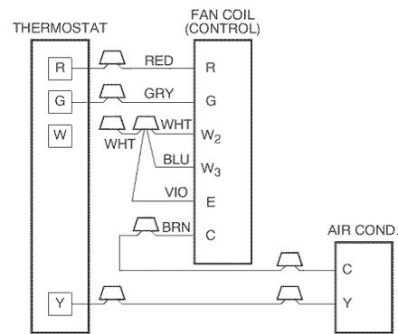
**Fig. 10 - Wiring Layout Air Conditioning Unit (Cooling Only)**
