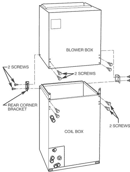
**Fig. 4 - Removal of Brackets on Modular Units**
