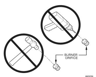
Fig. 60 - Burner Orifice
