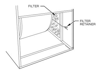
Fig. 26 - Filter Installed for Side Inlet
