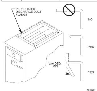
Fig. 24 - Duct Flanges
