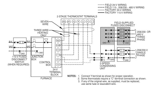
Fig. 32 - Typical Heating and Cooling Application Wiring Diagram 2-Stage Thermostat and Condensing Unit
