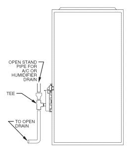
Fig. 46 - Example of Field Drain Attachment
