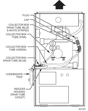
Fig. 7 - Alternate Upflow Configuration and Trap Location
