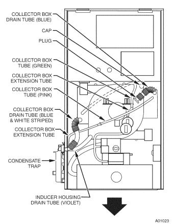
Fig. 8 - Downflow Tube Configuration (Left-Hand Trap Installation)
