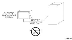
Fig. 33 - Disconnect Switch and Furnace
