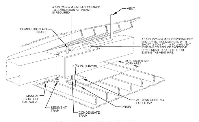
**NOTE:** LOCAL CODES MAY REQUIRE A DRAIN PAN UNDER THE FURNACE AND CONDENSATE TRAP WHEN A CONDENSING FURNACE IS INSTALLED ABOVE FINISHED CEILINGS.
