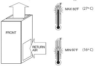
Fig. 4 - Return-Air Temperature
