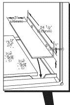
21-IN. (533mm) WIDE CASINGS ONLY: SUPPORT RODS (3) EXTEND 1/4" (6mm) ON EACH SIDE OF FILTER AND REST ON CASING FLANGE
