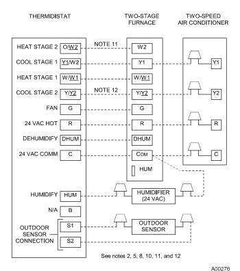
Fig. 51 - Two-Stage Furnace with Two-Speed Air Conditioner
