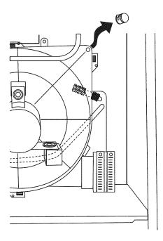
Fig. 48 - Inducer Housing Drain Tube Cap
