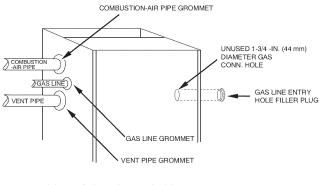
NOTE: PIPE GROMMETS AND ENTRY HOLE FILLER PLUGS ARE INCLUDED IN FACTORY-SUPPLIED LOOSE PARTS BAG
