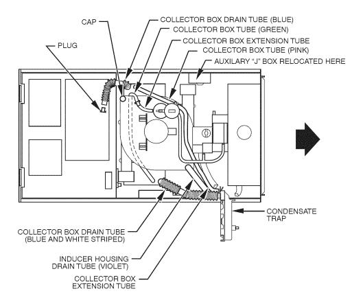
Fig. 13 - Horizontal Right Tube Configuration
