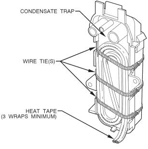
Fig. 47 - Condensate Trap Heat Tape
