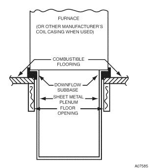
Fig. 21 - Floor and Plenum Opening Dimensions
