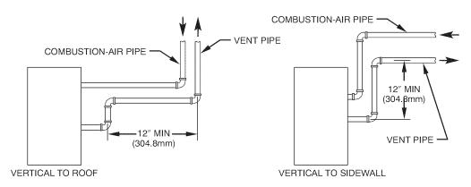
NOTE: A 12-in. (304.8mm) minimum offset pipe section is recommended with short (5 to 8 ft / 1.5 to 2.5M) vent systems. This recommendation is to reduce excessive condensate droplets.
