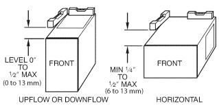
Fig. 14 - Proper Condensate Drainage
