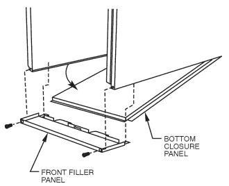
Fig. 28 - Removing Bottom Closure Panel
