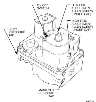
Fig. 58 - Redundant Automatic Gas Control Valve
