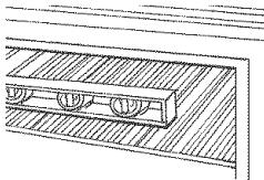
If the range is not level, pull range forward until the rear leveling leg is removed from the anti-tip bracket. Adjust the leveling legs up or down. Then slide range back into position. Check that leveling leg is engaged in anti-tip bracket.
