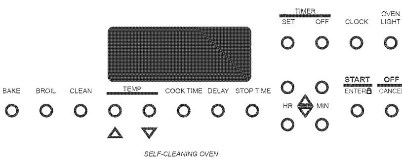
**24.** Check the operation of the oven burner. Push the "BAKE" pad and "Pre°F" will appear in the temperature display. Press the "Start/Enter" pad. A preheat time will count down. The oven burner should light in 50 to 60 seconds. This delay is normal. The oven safety valve requires a certain time before it will open and allow gas to flow.
