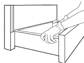
**30.** Insert storage drawer into slide rails on sides of drawer opening. Lift front of drawer slightly and push firmly to close drawer.
