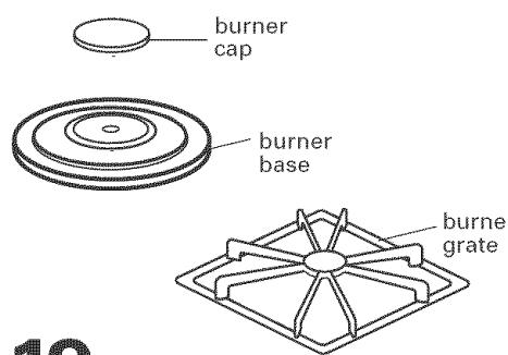
**19.** Remove cooktop burner caps and grates from parts package. Align notches in burner caps with pins in burner base. Burner caps should be level when properly positioned. Place burner grates over burners and caps.
