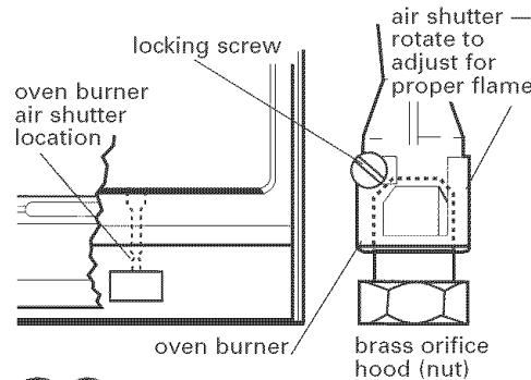
**26.** If the oven flame needs to be adjusted, locate the air shutter near the center rear of range. Loosen the locking screw and rotate the air shutter until the proper flame appears. Tighten locking screw.
