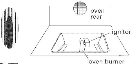
**25.** Check the oven burner for proper flame. This flame should have a 1/2" (1.3 cm) long inner cone of bluish-green, with an outer mantle of dark blue, and should be clean and soft in character. No yellow tips, blowing or lifting of flame should occur.
