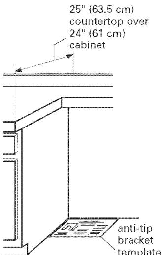
**8.** Place the anti-tip bracket template on the floor in the cabinet opening so that the left edge is against cabinets and the top edge is against the rear wall, molding or cabinet.
