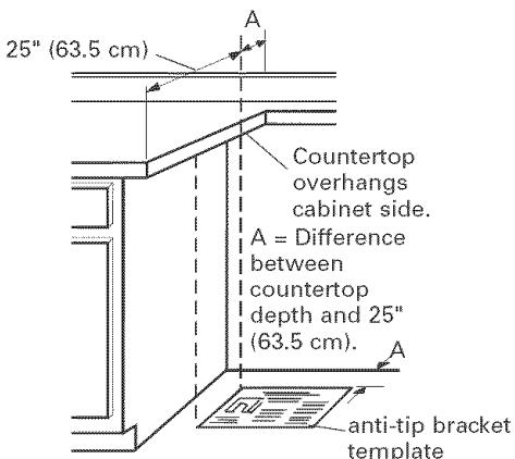
If countertop opening is deeper than 25 inches (63.5 cm), measure and mark a distance 25 inches (63.5 cm) in from front of countertop opening and align template with mark (or subtract 25 inches (63.5 cm) from countertop depth and add the difference to the corresponding dimension).
