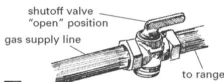
**F.** The supply line shall be equipped with an approved shutoff valve. This valve should be located in the same room, but external to the range, and should be in a location that allows ease of opening and closing. Do not block access to shutoff valve.
