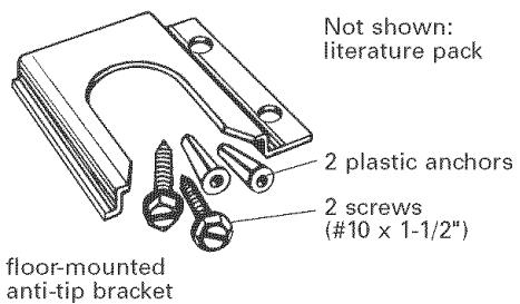
Brackets must be securely mounted to sub-floor. Thickness of flooring may require longer screws to anchor bracket to sub-floor. Longer screws are available from your local hardware store.
