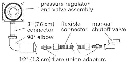
**14.** Assemble the flexible connector from the gas supply pipe to the pressure regulator, located in the lower left side of the storage drawer area, in this order: shutoff valve, 1/2" (1.3 cm) flare union adapter, flexible connector, 1/2" (1.3 cm) flare union adapter. Seal all openings in floor or wall wherever range is installed.
