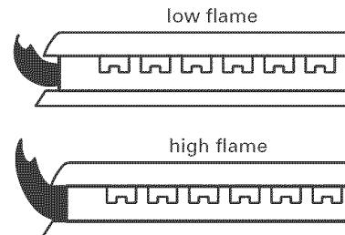
**22.** Adjust the height of top burner flames (some models). The cooktop LOW burner flame should be a steady blue flame approximately 1/4" (0.64 cm) high. It can be adjusted using the adjustment screw in the center of the valve stem. The valve stem is located directly underneath the control knob.
