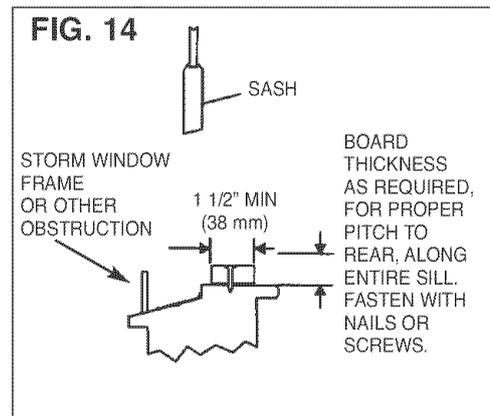
If Storm Window Frame must remain, be sure the drain holes or slots are not caulked or painted shut. Accumulated Rain Water or Condensation must be allowed to drain out.
