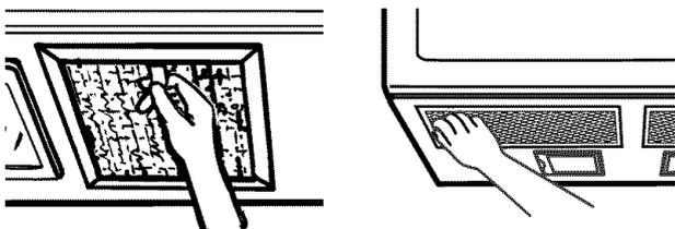
**8** Install grease filters. See the Owner's Manual packed with the microwave.
