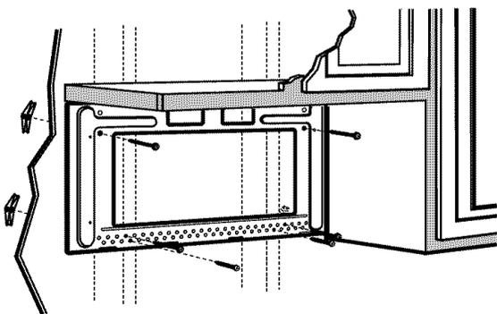
Attach the plate to the wall using toggle bolts. At least one wood screw must be used to attach the plate to a wall stud.
