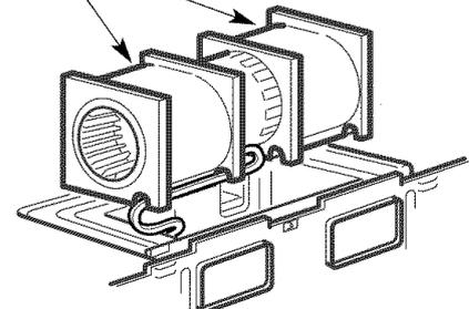
**NOTE:** Make sure wires remain routed in the grooves of the motor frame.
