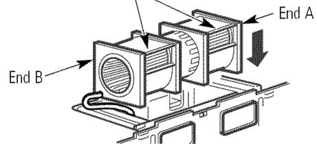
**CAUTION: Do not pull or stretch the blower unit wiring. Make sure the wires are not pinched.**
