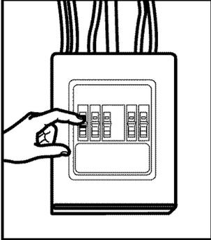
**CAUTION:** For personal safety, remove house fuse or open circuit breaker before beginning installation to avoid severe or fatal shock injury.
