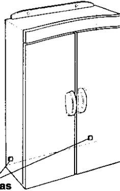
**8.** Check tops of doors for uniform vertical alignment. Wall irregularities may require shimming the back bottom corners of the cabinet away from wall to align the door tops.
