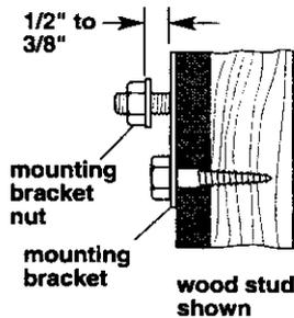
**6.** Space the mounting bracket nuts 1/2" to 3/8" away from mounting bracket.
