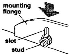
**7.** Lift clothes vitalizer up and slide keyhole slots over nuts. Lower vitalizer down onto mounting bracket studs and tighten nuts.
