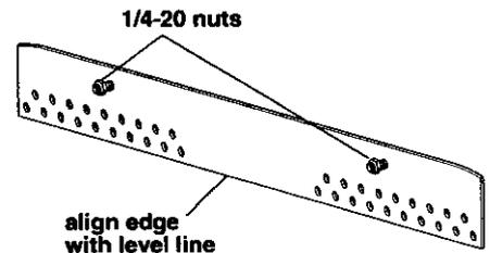
**4b.** Align the lower edge of the mounting bracket assembly with the level line. Select and mark a hole location on each side of the bracket that is closest to the center of each stud.
