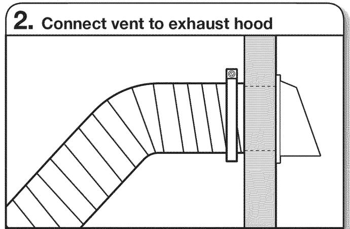
Vent must fit over the exhaust hood. Secure vent to exhaust hood with 4" (102 mm) clamp. Run vent to dryer location using straightest path possible. Avoid 90° turns. Use clamps to seal all joints. Do not use duct tape, screws, or other fastening devices that extend into interior of vent to secure vent, because they can catch lint.
