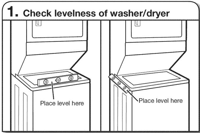
With washer/dryer in its final location, place a level on top edges of washer/dryer. Use side seam as a guide to check levelness of sides. Check levelness of front using lid, as shown. Rock washer/dryer back and forth to make sure all four feet make solid contact with floor. If washer/dryer is level, skip to step 2.
