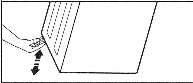
Tilt the washer/dryer forward. Move each of the 2 rear legs in an up-down motion to check the self-adjusting leveling legs for free movement. This is required for proper leveling. Gently lower the washer/dryer to the floor.
