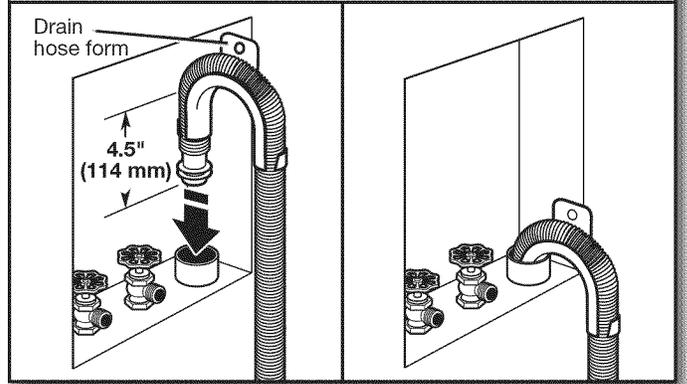
Place hose into standpipe (shown in picture) or over side of laundry tub.
