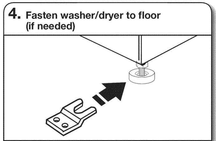
**For mobile home use:** Washer/dryers with gas dryers must be securely fastened to the floor.
