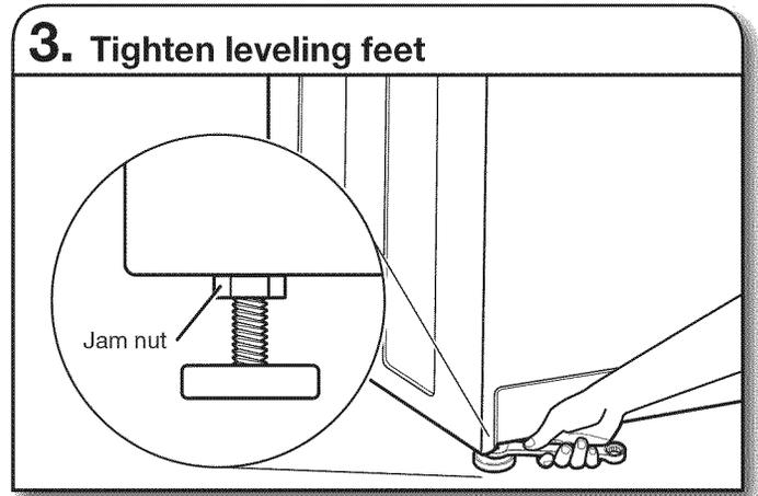
When washer/dryer is level, use a 9/16" or 14 mm open-end or adjustable wrench to turn jam nuts counterclockwise on leveling feet tightly against washer/dryer cabinet.
