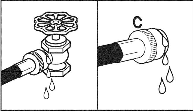
Turn on water faucets to check for leaks. A small amount of water may enter washer. It will drain later.
