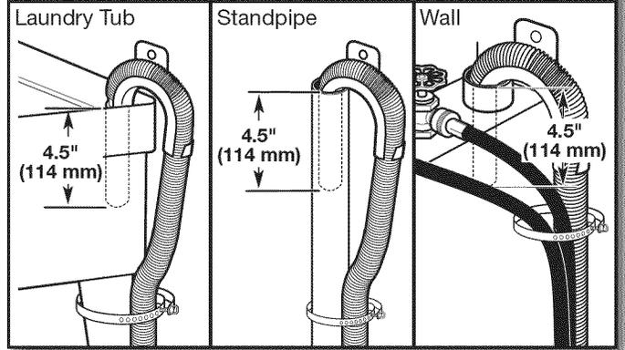
Secure drain hose to laundry tub leg, drain standpipe, or inlet hoses for wall standpipe with shipping strap removed earlier.
