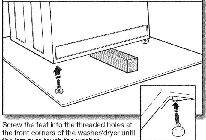
Screw the feet into the threaded holes at the front corners of the washer/dryer until the jam nuts touch the washer.
