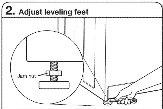
If washer/dryer is not level, use a 9/16" or 14 mm open-end or adjustable wrench to turn jam nuts clockwise on feet until they are about 1/2" (13 mm) from the washer/dryer cabinet. Then turn the leveling foot clockwise to lower the washer/dryer or counterclockwise to raise the washer/dryer. Recheck levelness of washer/dryer and repeat as needed.
