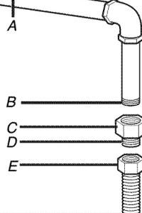
Install the adapter on the 1/2" rigid gas supply pipe using pipe-joint compound.
