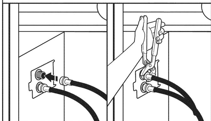
Attach hot water hose to the bottom inlet valve. Screw coupling by hand until it is snug. Use pliers to tighten couplings an additional two-thirds turn. Repeat with cold water inlet valve (top valve).
