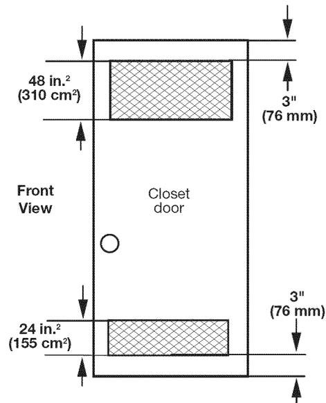
The spacing dimensions above are recommended for this washer/dryer. This washer/dryer has been tested for spacing of 0" (0 mm) clearance on the sides. Recommended spacing should be considered for the following reasons:
