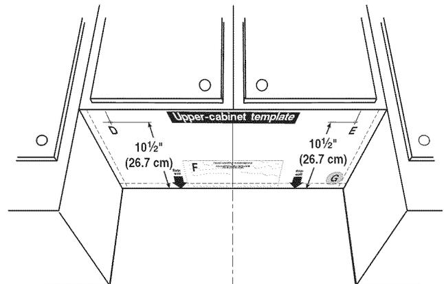
5. Cut the 1 1/2" (3.8 cm) diameter hole at the circular shaded area "G" on the template. This hole is for the power supply cord.
