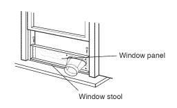
If the inner width of the window is between 28" (718mm) and 36.5" (927mm) inclusive.
