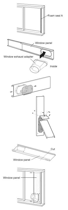
If the inner height of the window is between 28" (718mm) and 36.5" (927mm) inclusive.
