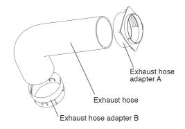
2 Attach the exhaust hose adapter B to the unit.
