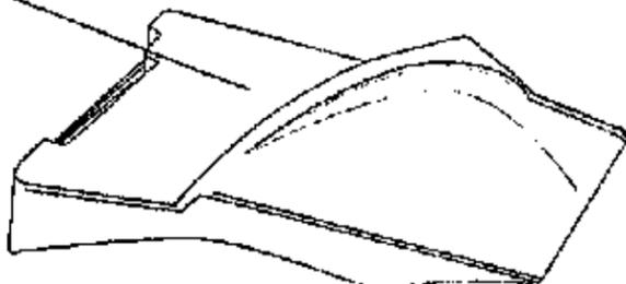
**Step 1. Lift rear flap, remove grass bag, if installed, and insert mulching plug.**
