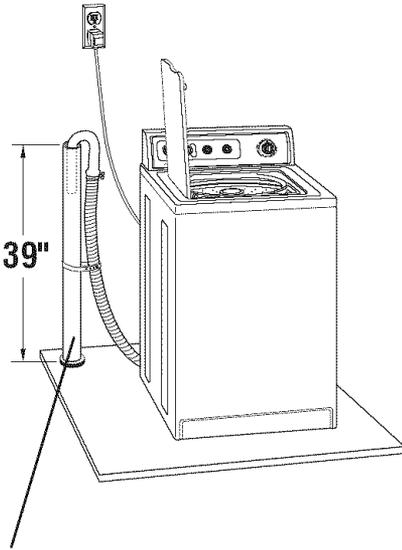
**Standpipe drain system:** Needs a two-inch minimum diameter standpipe with minimum carry-away capacity of 17 gallons per minute. Top of standpipe must be at least 39 inches above floor and no higher than 96 inches from bottom of washer.
