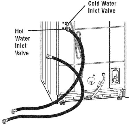
**STEP 3.** Attach the hose with the blue coupling to the cold water (top) inlet valve. Screw on coupling by hand. Make an additional two-thirds turn with pliers to tighten coupling. **DO NOT OVERTIGHTEN;** this could damage valves.
