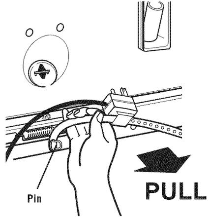
**STEP 4.** Cut the shipping strap about 16 inches from plug end. Look for the words "CUT HERE." Discard end with three cotter pins. Slide remainder of shipping strap from the electrical plug. You will use this to secure the drain hose.
