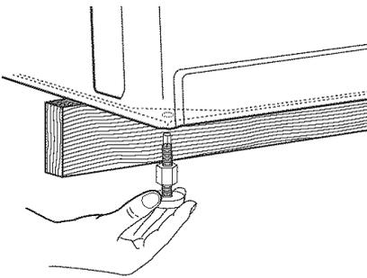
**STEP 4.** Tilt washer backward until front of washer is off the wood block. Remove wood block. Gently lower washer to floor.
