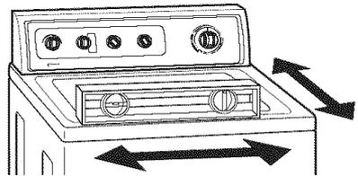
**STEP 7.** If washer is not level, prop up the front of the washer and adjust the legs up or down as necessary. Lower washer and reset self-adjusting rear legs (as in Step 6). Repeat Step 7 until the washer is level.
