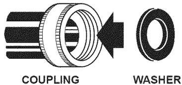
**STEP 2.** Attach the hose with the red coupling to the hot water (bottom) inlet valve. Attaching the red coupling first makes it easier to tighten connection with pliers. Screw on coupling by hand. Make an additional two-thirds turn with pliers to tighten coupling. **DO NOT OVERTIGHTEN;** this could damage the valves.
