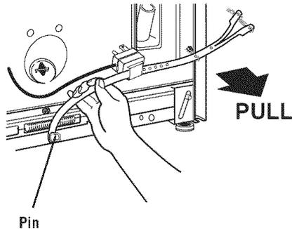
**STEP 3.** Pull firmly to remove the end of the shipping strap that remains pinned to the back of the washer. This will release the rear self-leveling legs.
