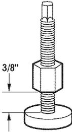
**STEP 3.** Screw leg into washer base by hand until nut reaches washer base. Repeat for other leg.
