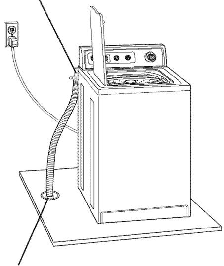
**Floor drain system:** Requires a siphon break, see chart below. A minimum carry-away capacity of 17 gallons per minute is required.
