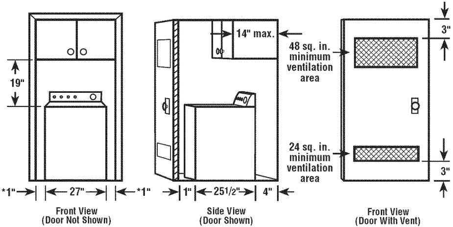
\*Additional clearance for wall, door and floor moldings may be required.
