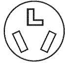
3-wire receptacle (10-30R)
