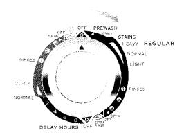
Rotate the control dial clockwise to the desired cycle.
