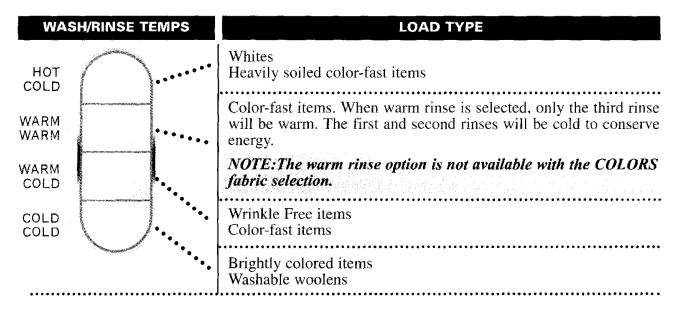
IMPORTANT: The washer features an automatic temperature control to provide a warm wash of approximately 105° F and cold wash of approximately 70° F.
