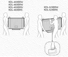
☐ When lifting or moving the TV, hold it firmly from the bottom. Place your palm directly under the panel.
