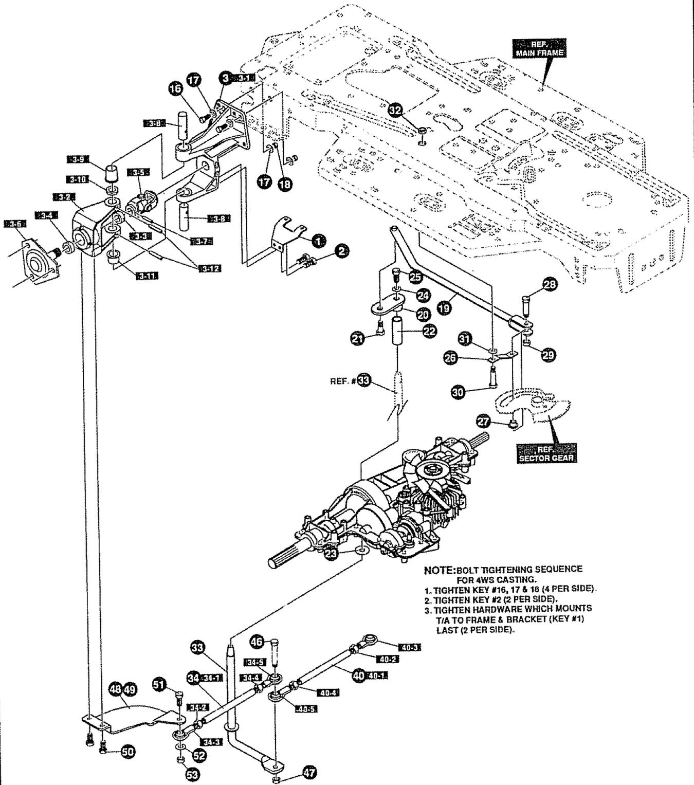
**NOTE: BOLT TIGHTENING SEQUENCE FOR 4WS CASTING.**
