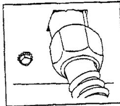
3. Connect the gas supply to the dryer. An additional fitting is required to connect the 3/4" female threaded end of a flexible connector to the 3/8" male threaded end on the dryer. Securely tighten the gas line fitting over threads.
