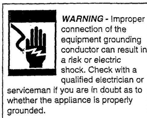
Do not modify the plug provided with the appliance - if it will not fit the outlet, have a proper outlet installed by a qualified electrician.
