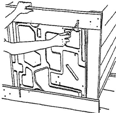
3. Loosen the leveling locking nuts and install the vinyl feet.
