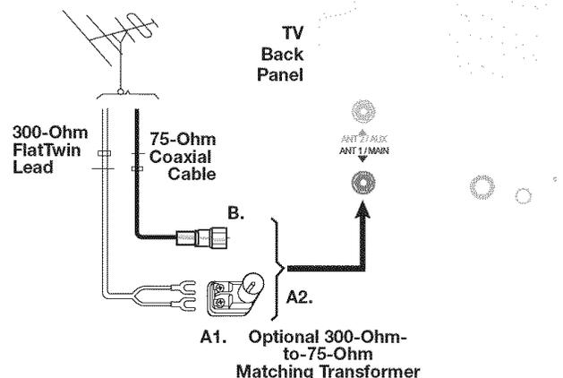
Figure 6. Connecting a Single Antenna Lead
