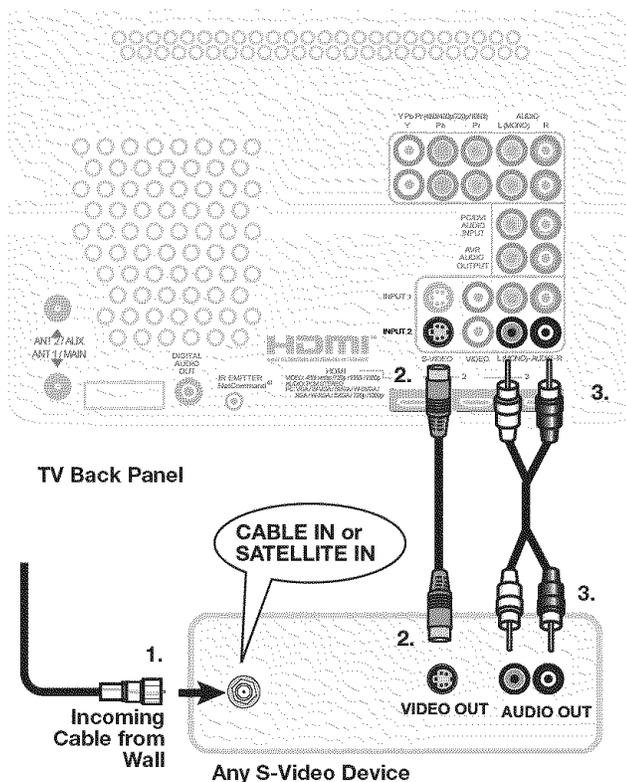
Figure 2. Connecting a device with S-Video
