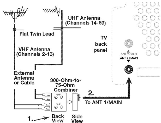
Figure 5. Connecting separate UHF and VHF Antennas
