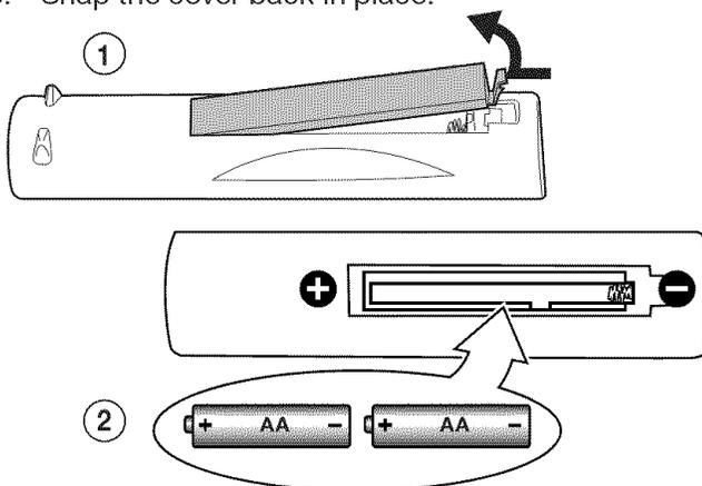
The remote control requires two AA alkaline batteries.
