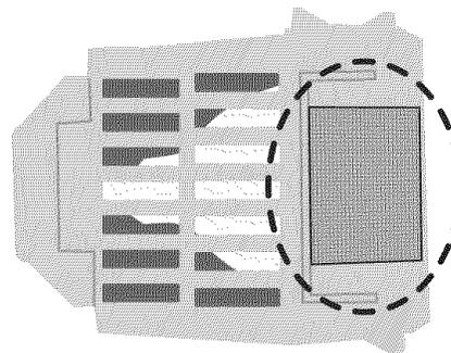
Keep lamp cartridge horizontal and remove dust from the mesh filter using a soft dry brush or vacuum cleaner.
