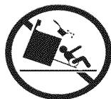
To reduce the risk of tipping, the wall oven must be secured by properly installed anti-tip bracket provided with the wall oven. Refer to the Installation Instructions for proper anti-tip bracket installation.
