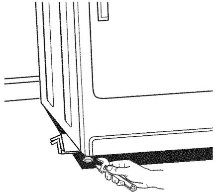
**NOTE:** It may be necessary to level the dryer again after it is moved into its final position.
