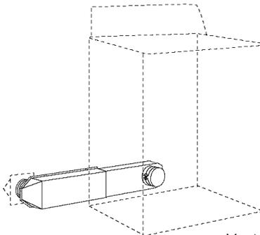
Vent system with one periscope (2-inch clearance)
