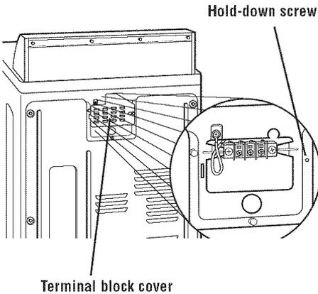
**STEP 3.** Attach a  $\frac{3}{4}$ -inch, U.L.-listed strain relief to the hole below terminal block opening. Strain relief should have a tight fit with dryer cabinet and be in a horizontal position. Put the power supply cord through the strain relief.
