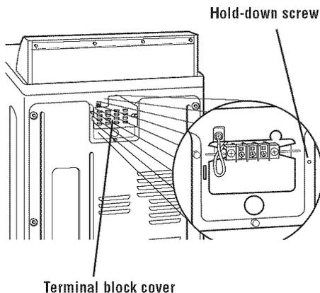
**STEP 5.** Connect neutral grounding wire and the neutral wire (white or center) of power supply cord under the center screw of terminal block.
