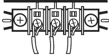
**STEP 7.** Connect the other two wires to outer terminal block screws. Use the same method described in STEP 6.
