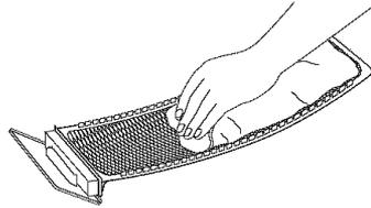
**STEP 3.** Push the lint screen firmly back into place.
