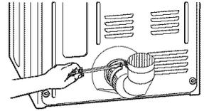
**STEP 4.** Connect vent to elbow. Tape the joint with duct tape. Tighten clamp.
