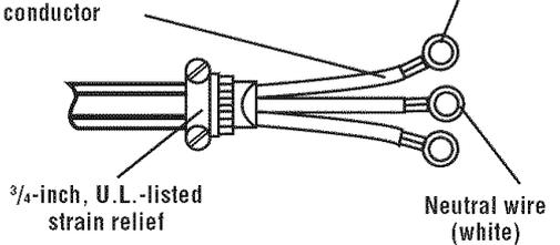
Spade terminals with upturned ends (OR ring terminals)
