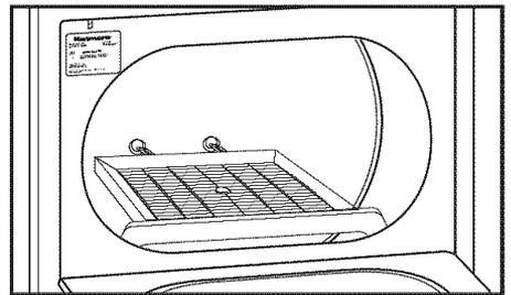
**STEP 3.** Place wet items on top of the dry rack. Allow space around items for air to circulate. The rack does not move, but the drum will rotate. Make sure items do not hang over the edges or between rack grill.
