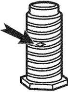
**STEP 4.** Start to screw the legs into the holes by hand. Use a wrench to finish turning the legs until diamond marking is no longer visible. This is when we recommend you start checking the dryer for levelness. Further adjustment may be necessary.
