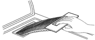
**STEP 2.** Roll lint off the screen with your fingers. Do not rinse or wash screen to remove lint. Wet lint is hard to remove.
