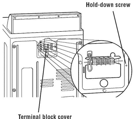
**STEP 3.** Attach a 3/4-inch, U.L.-listed strain relief to the hole below terminal block opening. Strain relief should have a tight fit with dryer cabinet and be in a horizontal position. Put the direct wire cable through the strain relief.
