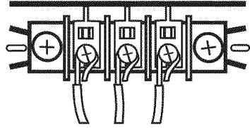
**STEP 5.** Connect the other two wires to outer terminal block screws using the same method(s) described in STEP 4a. Securely tighten all electrical connections.
