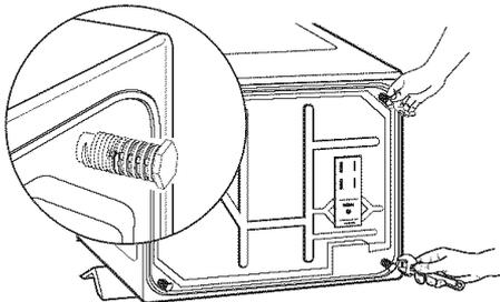
**STEP 5.** Stand the dryer up and move it close to its final location. Leave enough room to connect the exhaust vent.
