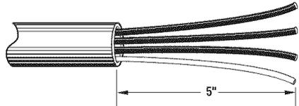
**STEP 1b.** Cut 1½ inches from the three remaining insulated wires. Strip insulation back 1 inch. Shape the end of each wire into a "U" shaped hook.
