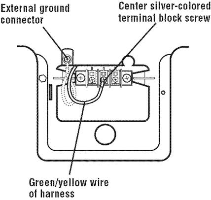
**STEP 5.** Connect neutral grounding wire and the neutral wire (white or center) of direct wire cable under the center screw of terminal block.
