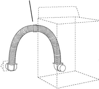
Vent system installed over-the-top with standard elbows
