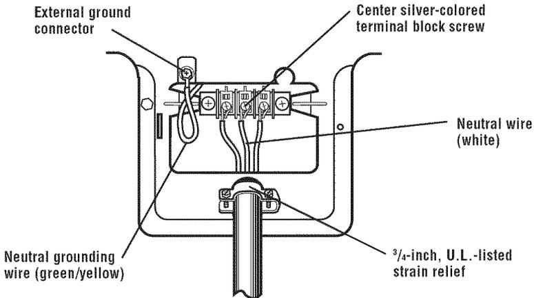
**3-Wire Connection with Direct Wire and Frame-Grounding Conductor**
