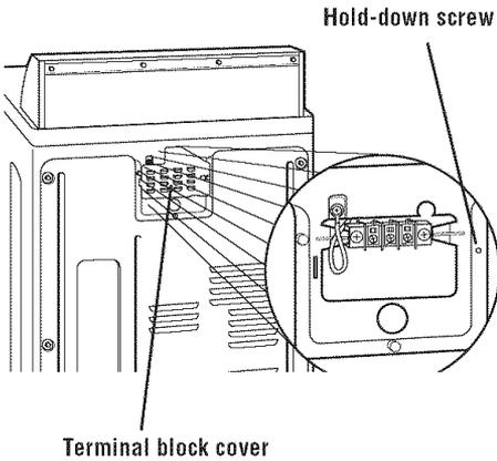
**STEP 4a.** Place the hook-shaped end of the wire over the terminal block screw. The open side of the hook should face to the right. Squeeze hook end of wire together to form a loop.
