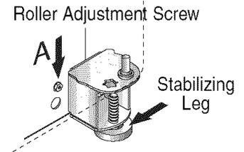
6. Turn adjustment screws **(A)** counterclockwise to allow the full weight of the refrigerator to rest on the stabilizing legs.
