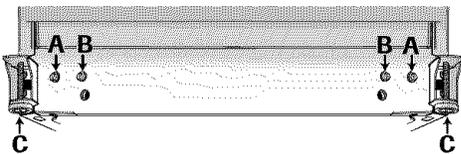
3. Select models also have rear adjustment screws **(B)**. Using the hex head driver, turn each of these adjustment screws **(B)** to raise or lower the rear of the refrigerator.
