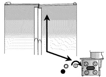
7. If required, correct rocking of refrigerator by turning rear adjustment screw clockwise to raise rocking corner. If doors are uneven, do the following:
