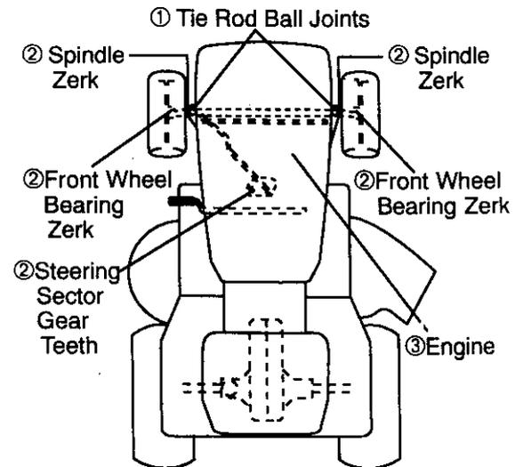
① Spray Silicone Lubricant (Move Boots to Lubricate)
