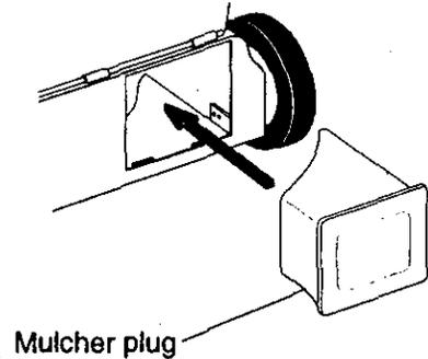
**CAUTION:** Do not run your lawn mower without mulcher plug in place or approved clipping deflector or grass catcher in place. Never attempt to operate the lawn mower with the rear door removed or propped open.
