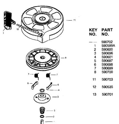
DESCRIPTION Recoil Starter Spring Pin (Incl. 4) Washer Retainer Washer Brake Spring Starter Dog Dog Spring Pulley & Rewind Spring Ass'y. Starter Housing Ass'y. (40 degree grommet) Starter Rope (98" X 9/ 64" dia.) Starter Handle
