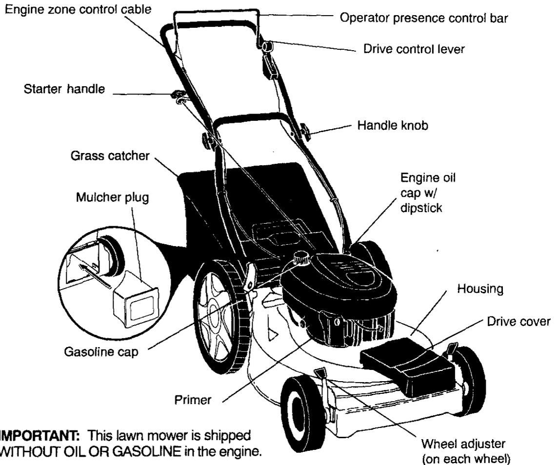
**IMPORTANT:** This lawn mower is shipped WITHOUT OIL OR GASOLINE in the engine.
