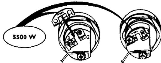
8. The wire removed from terminal 2 has a looped end. It must remain looped and now be placed (as shown) on top of the buss bar, over the opening of terminal 2, and secured using the remaining screw.
