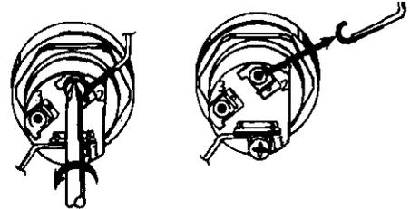
7. The buss bar is labeled 5500 W. Place the buss bar over terminals 2 and 3 with the 5500 W visible. Install the extra screw provided into terminal 3.
