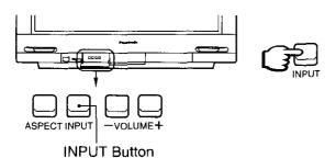
Press the INPUT button to select the input video signal to be played back from the equipment such as a VCR which has been connected to the Monitor.
