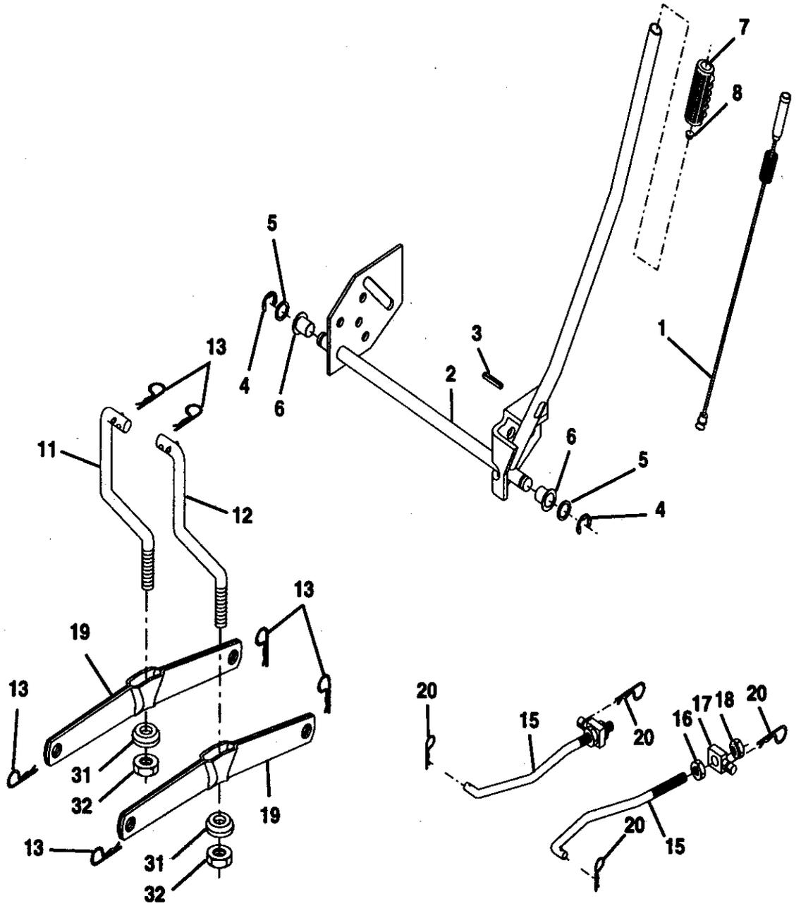
**LIFT ASSEMBLY****TRACTOR -- MODEL NUMBER 917.271060**
