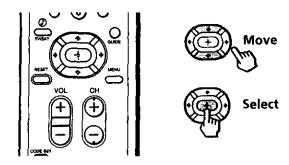
The supplied remote control has "arrow" buttons  $(\blacklozenge, \blacklozenge, \spadesuit, \spadesuit)$  which allow for movement of the on-screen  $(\blacktriangleright)$  cursor. Pressing on the outer buttons will cause the cursor to *move* in the corresponding direction. Pressing the center button  $(\clubsuit)$  will *select* the item.
